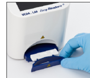
Figure 21 : Load the pipetted assay device into the rapid test holder, and insert the holder into the analyzer.
