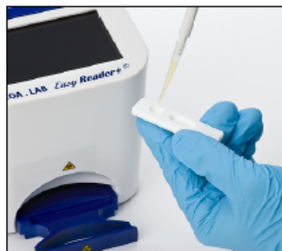
Figure 20 : Use a manual pipette to apply the amount of specimen that the package insert of the assay device requires into the sample well of the assay device.
