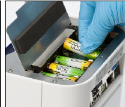
Figure 6: When you insert the batteries, always pay attention to the polarities
